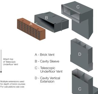
This product should be used in conjunction with other products from the brick ventilation range to provide a complete through wall ventilation system.
