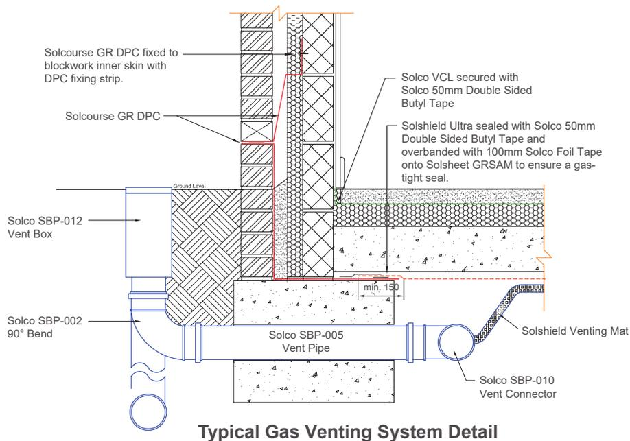
Typical Gas Venting System Detail
