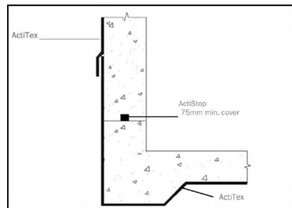
Figure 1.19 – Slab/wall with kicker
